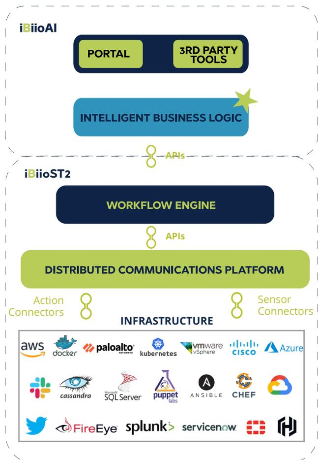
Figure 1 - iBiiio Platform Architecture
